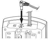
4. Route the adapter's cord through the strain relief slot on the bottom of the base.
